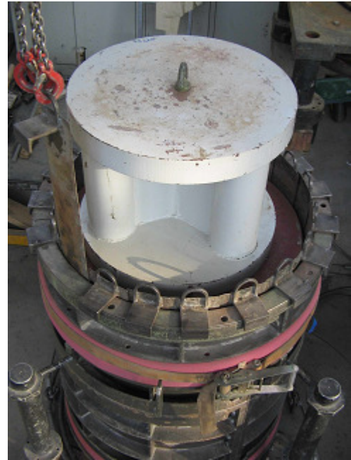
Fig. 9: Sample in the sample former after compaction under static load, with the protective metal strips being removed one by one before mounting of the top plate
