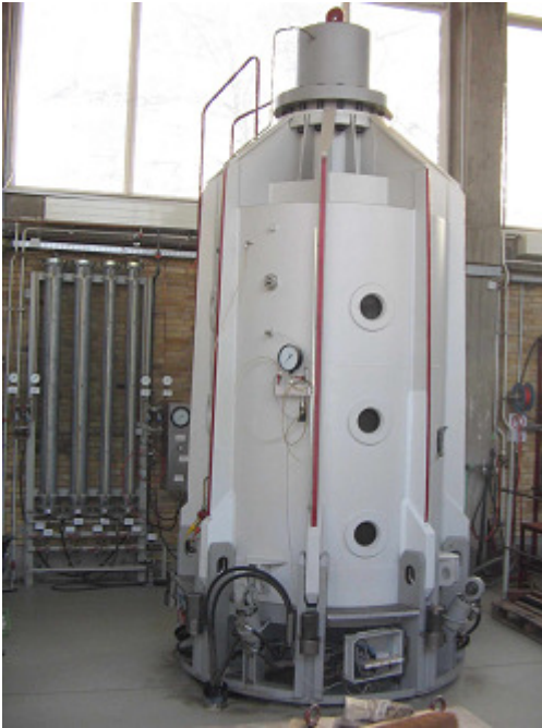
Fig. 11: Large scale triaxial cell for tests on H = D = 800 mm specimens (cell pressure up to 20 bar)
