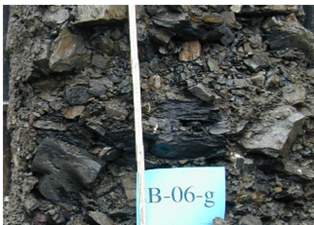
Fig. 15 View on inner section of a specimen after triaxial testing
