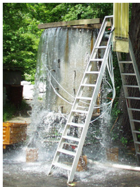
Fig. 17: Water permeability test on rockfill (Diameter of specimen: d = 1200 mm)
