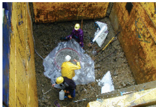
Fig. 8: In situ density tests with the water displacement method
